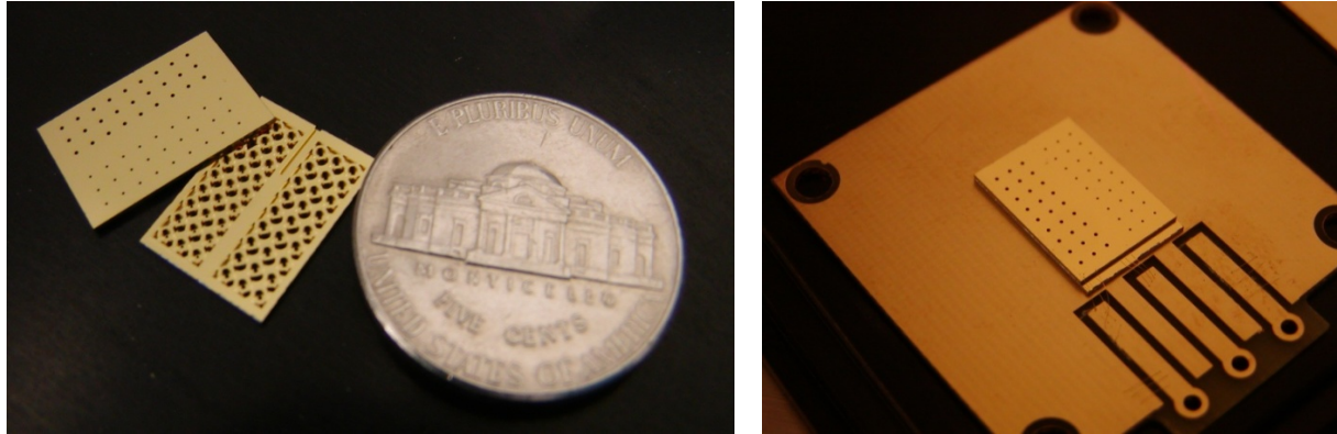
Figure 23 Left: Optical image of the two symmetrical \mu CIT array half-structures before bonding. Right: Complete \mu CIT array obtained after bonding the two arrays of halfCITs mounted on an Au-coated PCB substrate.
